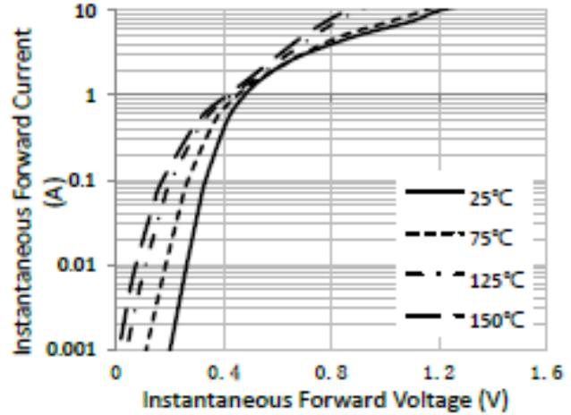
Figure 2. Typical Instantaneous Forward Characteristics (SGP0120SD thru SGP0140SD)
