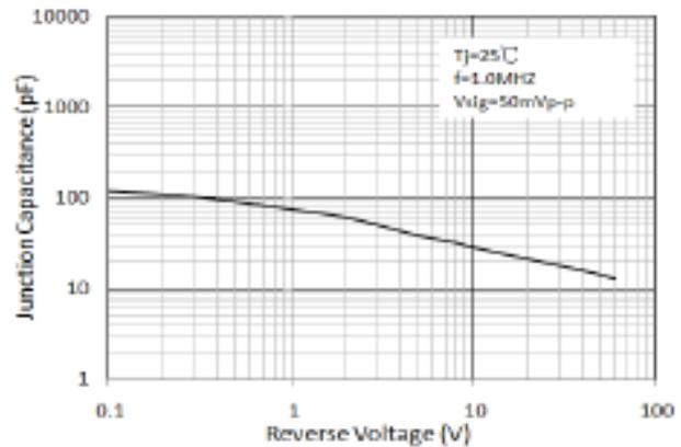
Figure 6. Typical Junction Capacitance
